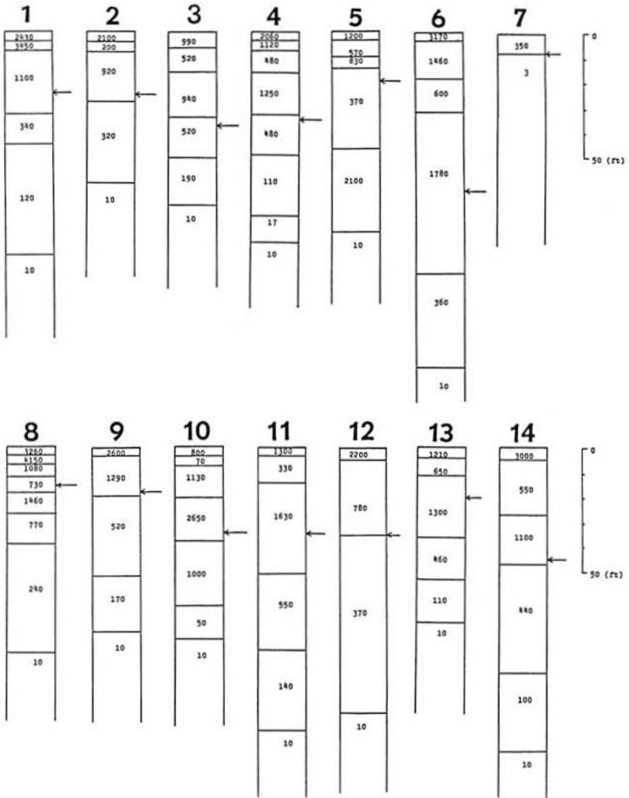
Figure 3: Computer generated resistivity layer models based on field sounding curves. Arrows indicate sealevel. Discussion in text.
