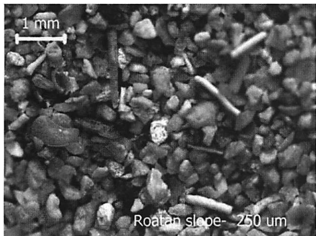
Figure 7. Mean and mode grain size of slope showing primary sediment type; spicules, forams, and intraclasts.
